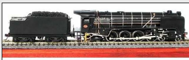
D24 – These models are hand built on a Mehano chassis to 16.5mm gauge and come pre-fitted with Kadee couplers. They feature constant current lighting and a sub miniature plug to connect the locomotive to the tender.
