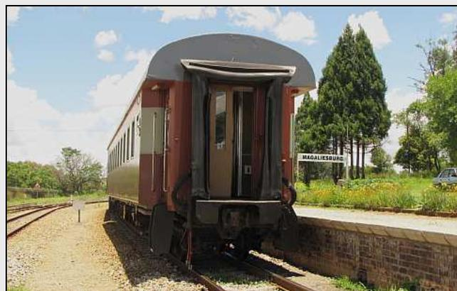
D12 – A coach-end from ballast height, plus 6ft2. Notice a rarely-intact feature on the aging mainliners – the drip-strip on the upper gangway bellows tube. Notice the three cables hanging. Two of them are mains power (2Ph and 1Ph + N) while the smaller red one is for the newly installed PA system, which is reported to be working well.
