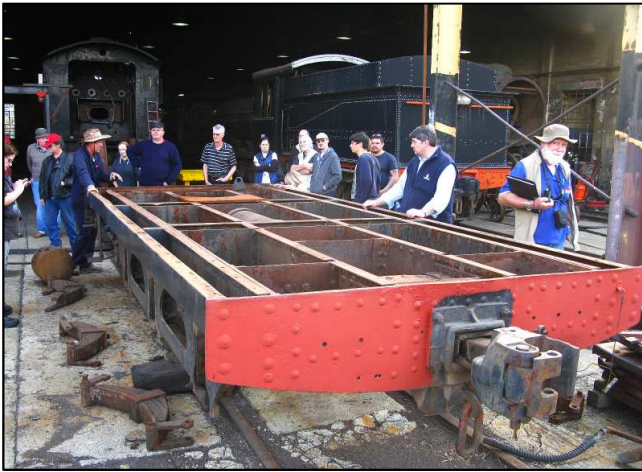
P01 - Our first RED tour group are being shown what a late 19 th century tender frame looks like.
