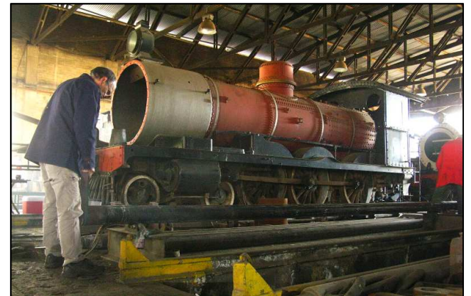
P04 - With Class 6A 473 'Charlotte' in the background, Danie Gouws de-scales the front end of one of 15CA 2056's new boiler flues with a strip of emery cloth.
