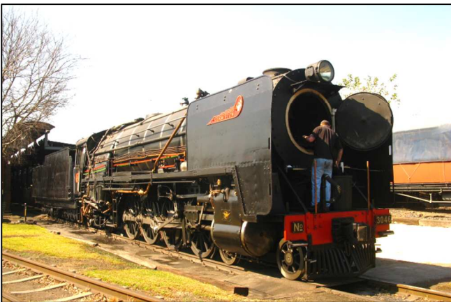
P05 - 15F 3046 Smokebox washout in progress. This was a young people's project today done by Aidan and Kevin.
