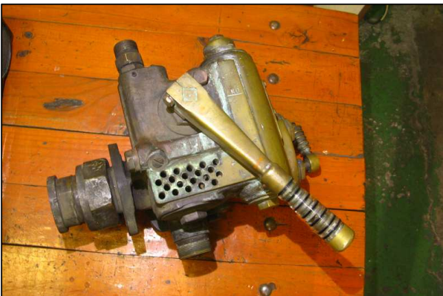
P07 - Brake Vacuum Ejector on its way back to FotR and 15F 3052's faulty unit to be returned.
