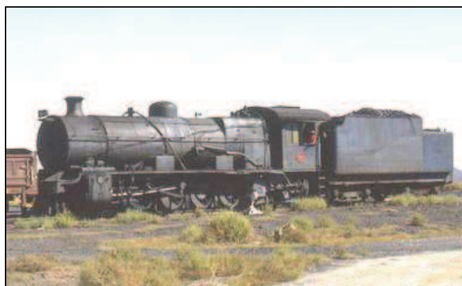
Lil' Susie used to look like this – note the square-topped Belpaire type firebox. This is an original Class 12A No.1526 running her last years as a shunter at De Aar in 1979. (Pic by Malcolm Best.)
